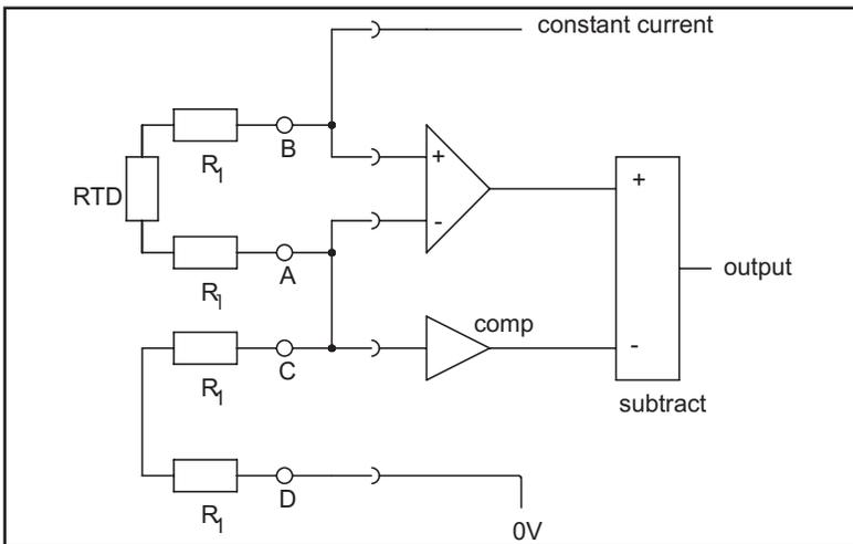
Figure 7.9 Connections for 4 Wire Compensated RTDs
