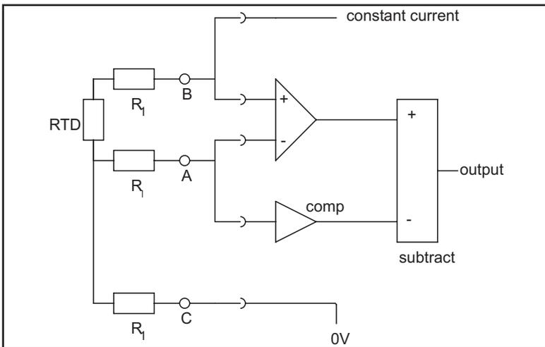
Figure 7.7 Connections for 3 Wire RTDs
