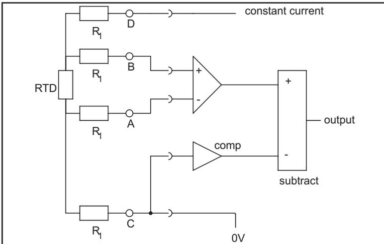
Figure 7.8 Connections for 4 Wire RTDs
