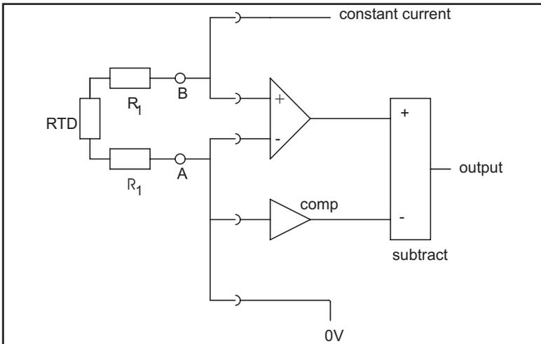
Figure 7.6 Connections for 2 Wire RTDs
