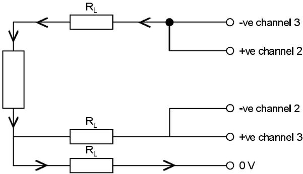
Figure 2.7 Three Wire Connection to Channel 2
