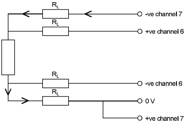
Figure 2.8 Four Wire Connection to Channel 6
