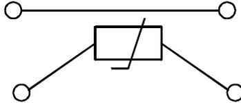
*Figure 2.5 Four Wire Compensated Configuration*
