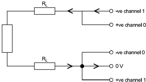
*Figure 2.6 Two Wire Connection to Channel 0*
