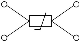
*Figure 2.4 Four Wire Configuration*
