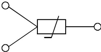
*Figure 2.3 Three Wire Configuration*
