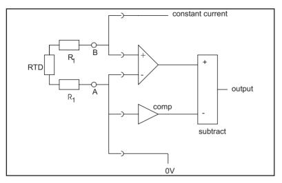
Figure 7.6 Connections for 2 Wire RTDs
