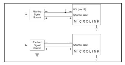
Figure 7.1 For floating signals you need to connect one end of the signal to the 0 V input on pin 19
