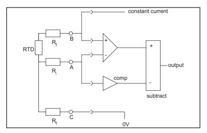
Figure 7.7 Connections for 3 Wire RTDs
