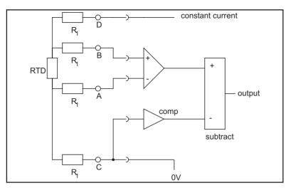
Figure 7.8 Connections for 4 Wire RTDs
