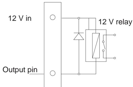
Figure 2.2 Microlink 840 Relay Drive Output
