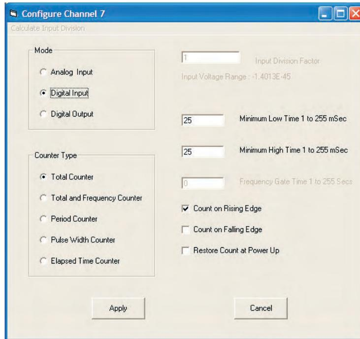
Figure 3.3 Configuring a Digital Input Channel
